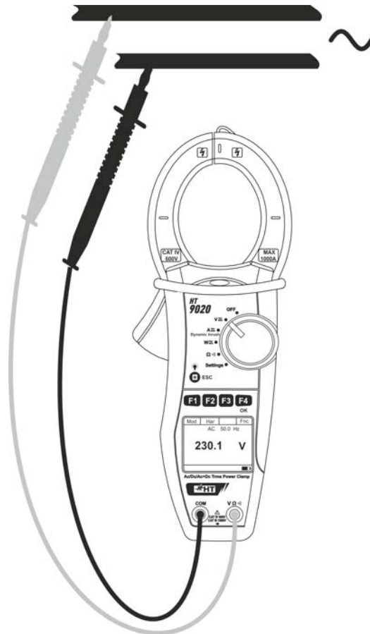
Fig. 6: AC/AC + DC voltage measurement
