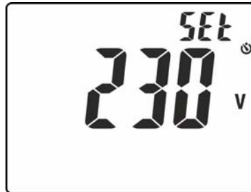
Fig. 6: Setting the rated voltage in Loop measurement
