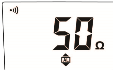
Fig. 33: Setting of alarm thresholds in resistance measurement
