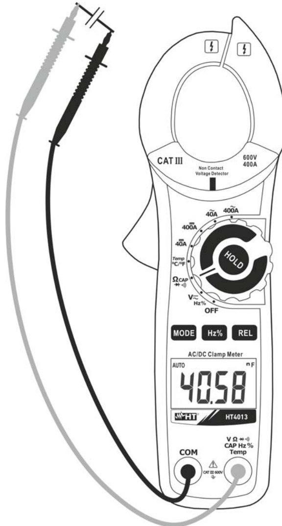
Fig. 6: Use of the clamp for capacitance measurement
